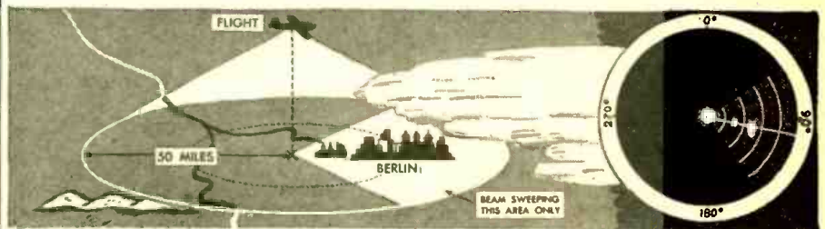
25 MILES FROM TARGET. SECTOR SCAN IN OPERATION, AIRCRAFT HEADING IS NOW 100°.
